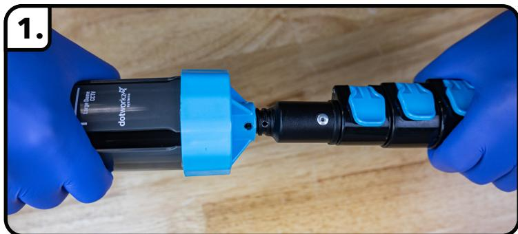
Fasten cleaning head to pole tightly.
