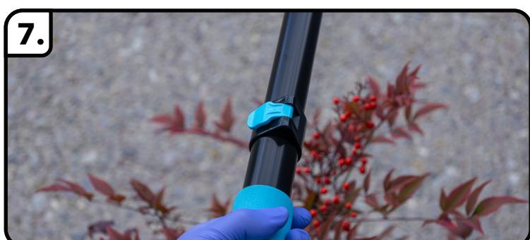
Close blue pole latches completely (to avoid pole collapse when in use).
