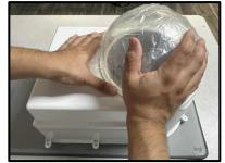
B. If properly bonded, the dome lens should not have any movement nor visible air gaps between the VHB seal and the lens flange.
