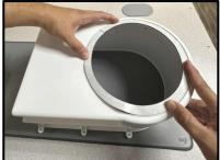
B. Remove the white liner in the VHB seal to expose the adhesive and press the dome lens into it. Remember to maintain proper center alignment while installing the dome lens.
