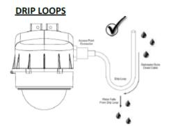
Always Create a Drip Loop for all Cables or Conduit Entering
