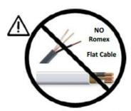
Use Round Cable Only with provide Cable Gland Port Seal
