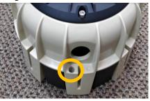
Now Install Microphone element: There should be a loose piece of black heat shrink around neck of microphone wire (set it aside loose heat shrink for now, as loose heat shrink jacket is for shimming into hole later, around mic element).
