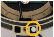
Now Insert new Cable gland port that is on mic assembly as shown lower left, then re-install tightening retainer nut.
