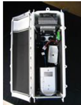
S-Type COOLDOME after power & camera installation- typical
