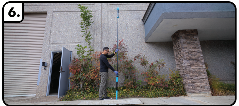
Extend (or retract) pole to desired height (only when pole is vertical).
