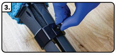
Loosen set screw, select desired cleaning mode, tighten set screw.
