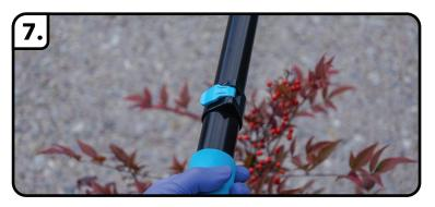
Close blue pole latches completely (to avoid pole collapse when in use).
