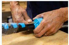
6) Press down both bent legs firmly to securely detail & set cotter pin firmly in place.
