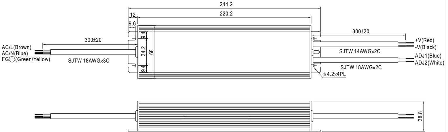
※ IP67 rated. Output constant current level can be adjusted through output cable by connecting a resistor between ADJ1 and ADJ2.
