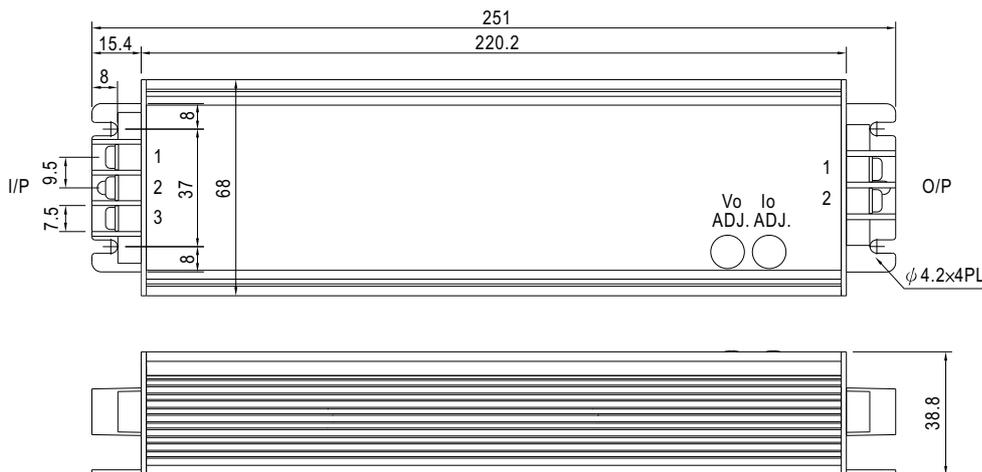
AC Input Terminal Pin No. Assignment
