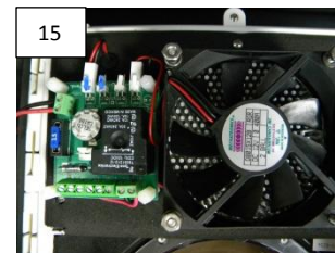
13) Re-Install washers & Nuts on fans first by finger tight, then 1/4 turn-or-less after contact with fan surface. Thread lock is advised. 14&15) Re-Install all wires, observe proper polarities and original wire locations- from nearest side view, Dotworkz uses red wire (+) on right convention/ black (-) on left for each terminal. Confirm with PCB polarity markings. External Fan Plugs in to either of two fan headers that are nearest to hinge. Internal fan headers on PCB are nearest to fan on Cold Sink. Re-Install Cooler Wires from Cold Sink on terminals marked S+TEC (Switched Thermal Electric Cooler) observing Positive/ Red farthest to right. Re-Install camera power cables to terminal blocks observing polarity and markings on PCB 16) Re-Install nylon PCB Fasteners. 17) Re-Install Terminal block and cable management fasteners (reverse of illustrated items #1 & #2) 18) Always test Polarity and confirm voltage of power coming into D2 from external step down power supply - to confirm Low Voltage 12 VDC. 12 VDC Only- Red to Red Positive (+), Black to Black Negative (-) Re-install power wires from low voltage input power from external power supply:
