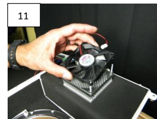
9) Unscrew four #6 nuts & washers for fan with 5/16" nut driver 10&11) Remove old fan 12) Replace with new fan, Install wire leads nearest to PCB side
