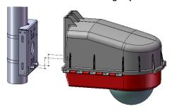
3) Then install last two 3/8" dia. x 3/4" long bolts into upper mount holes on D2 & thread into inserts on EZ
