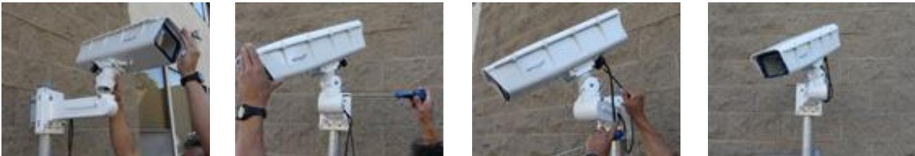
Attach housing to arm as shown, tighten screws evenly but firmly on both sides of housing. Adjust housing to desired position using both pan & tilt adjustment fasteners and tighten all bolts evenly & securely, so housing is pointing into final position.
