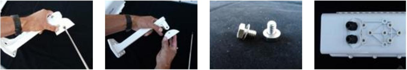
Remove Tilt bracket by unscrewing two side screws with #2 Phillips screwdriver as shown, set aside screws that were removed. Locate two ¼"-20 x ½" bolts & washers provided in hardware pack for mount & mate to two rear-most threaded Inserts on bottom of S-Type.
