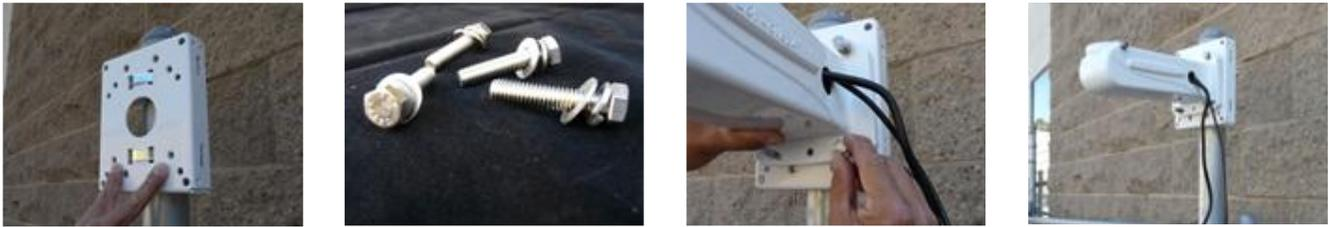
Pre-Install EZ-Lock Pole Mount #BR-MPM1 (sold separately) by following Instructions detailed in Installation Guide provided with pole mount bracket. Pole Mount requires user supplied stainless steel strapping to secure Pole Mount Bracket to the pole, strapping into final desired position. Locate four (4) 5/16"-18 x 1.5" Hex bolts & washers provided with EZ-Lock, and securely fasten base of S-Type Strong-Arm to Bracket.
