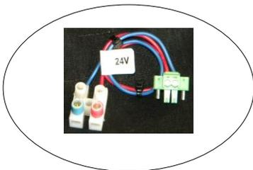
Locate Green Plug on Chassis Then Unplug from panel mount socket, then push aside
