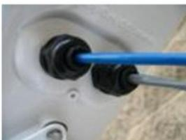
Be sure to tighten cable gland seals to assure a weather tight seal. Gently but firmly tighten four enclosure cover screws to fully seal enclosure.
