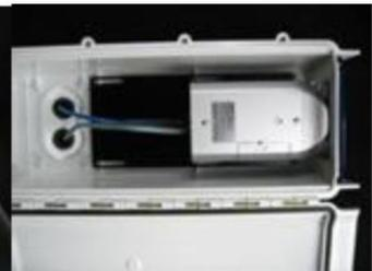
Re-install camera plate into S-Type, placing camera lens close to enclosure lens. For cameras that have adjustable focal lens', allow enough room for lens clearance. Re-install & Tighten all mounting plate screws.
