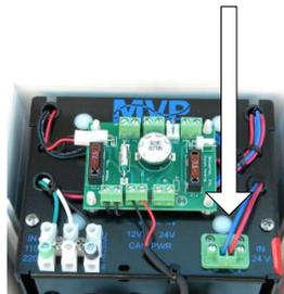
Then insert similar Plug on 24V Bypass Cable Tighten screws on plug to secure
