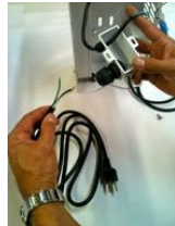
Remove High Voltage input Wiring Box by removing two machine screws that fasten it to metal bracket
