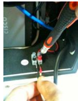
Using a small flat blade screw driver, secure wires to color coded terminals as shown
