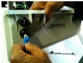
Feed Cat5e/ 6e cable thru port as shown
