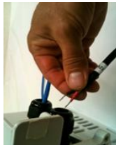
First feed thru round port on metal bracket
