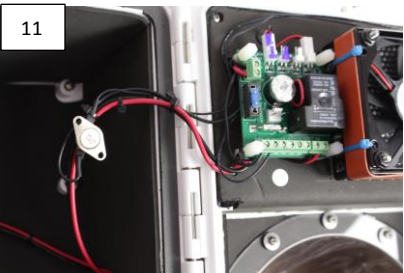
10-12) Use Provided Cable Wire Zip to secure Thermostat to wires, keeping away from heater or cooler components to sense air temperature in housing, keeping away from PCB, hinge & seals, so as to keep clear of closing surfaces. Point metal face of thermostat toward inside of housing to best sense air temperature
