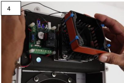
4 & 5) Install Heater Bracket over Cooler Cold Sink with wire leads from heater oriented to back of D2, and the four #6 threaded studs aligning with holes.
