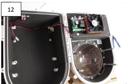
10-12) Use Provided Cable Wire Zip to secure Thermostat to wires, keeping away from heater or cooler components to sense air temperature in housing, keeping away from PCB, hinge & seals, so as to keep clear of closing surfaces. Point metal face of thermostat toward inside of housing to best sense air temperature
