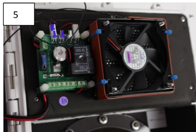
4 & 5) Install Heater Bracket over Cooler Cold Sink with wire leads from heater oriented to back of D2, and the four #6 threaded studs aligning with holes.
