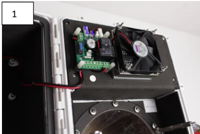
1) Older COOLDOME models have bare Cooler as shown in figure 1, and are ready to install heater
