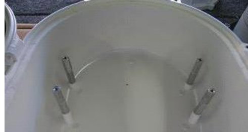
Picture represents standoff location & orientation. Height of standoffs will vary depending on camera used.
