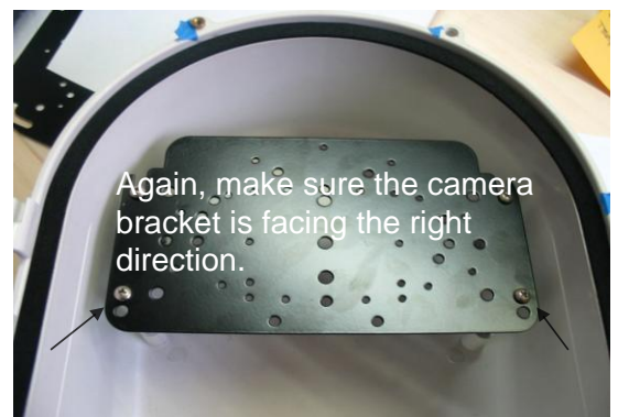
Picture represents camera bracket orientation & how it is secured. Don't forget to mount your camera to the D2 camera bracket based on instructions.
