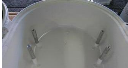
Picture represents standoff location & orientation. Height of standoffs will vary depending on camera used.
