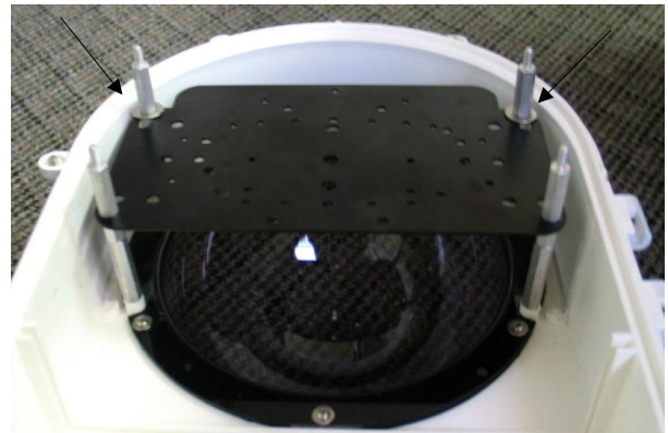
Picture represents camera bracket orientation & how it is secured. Don't forget to mount your camera to the D2 camera bracket based on instructions.
