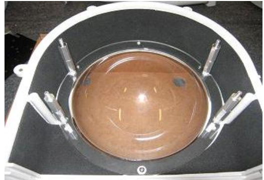
Picture represents standoff location & orientation. Height of standoffs will vary depending on camera used.
