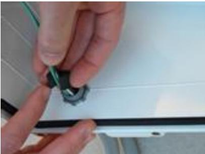
2) Open Vent Stop Plug and install over wire.
