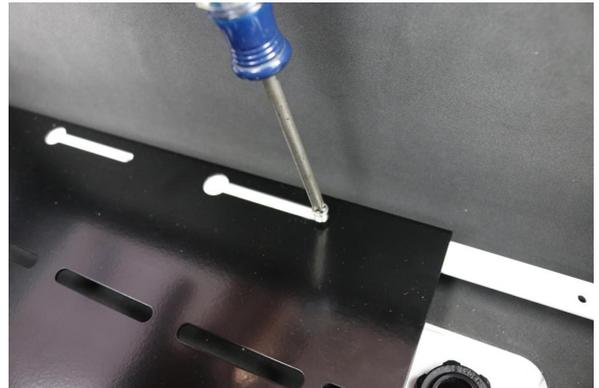
Remove the 4 screws on the camera mounting plate and set aside.
