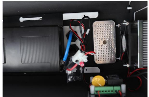
Place the humidity removal pack (included) near the back of the housing on the insulation pad.
