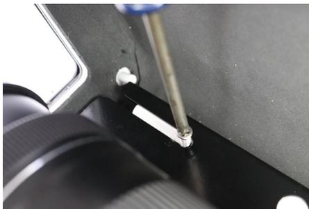
Locate the 4 camera mounting plate screws and loosely fasten mounting plate to housing.
