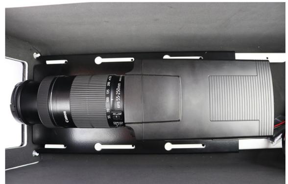
Check to make sure lens is not touching the glass. If it is, simply slide the camera mounting plate backward. Tighten screws to secure position.
