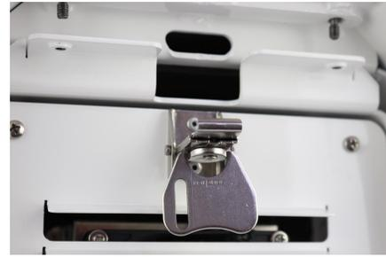
Loosen the lockable latch on the back side of the housing.
