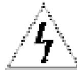
The lightning bolt with an arrowhead symbol, within an equilateral triangle, is intended to alert the user to the presence of non-insulated "dangerous voltage" within the product's enclosure that may be able to cause electrical shock to persons.
