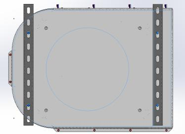
Pre-mount UniStrut to ceiling @ 21.5" O.C. Spacing oriented as shown above & below, then place Spring Clamping Nuts into UniStrut centered & spaced @ 12" O.C. into UniStrut channel. Open Bottom Clamshell of BRZ12 Aluminum outer shell to Access front & Back Mount Holes. Lift BRZ12 into place & use provided 3/8" bolts & washers to Secure BRZ12 to UniStrut Nuts & ceiling structure.
