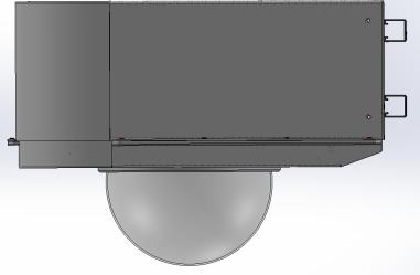
Pre-mount UniStrut to wall @ 5.5" O.C. Spacing oriented as shown above & below, then place Spring Clamping Nuts into UniStrut centered & spaced @ 10" O.C. into UniStrut channel. Open Bottom Clamshell of BRZ12 Aluminum shell to Mount & Access Rear Holes, while lifting BRZ12 Housing into place, & anchor to UniStrut Spring Nuts using provided 3/8" bolts & washers to Secure BRZ12 to ceiling structure.
