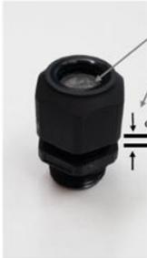
An UNSEALED Cable Gland has Rubber Seal below the top / outer face of the Compression Nut, & a GAP between the bottom of Compression Nut and the wrenching nut Body of the Cable Gland
