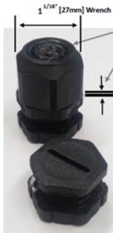
A SEALED Cable Gland has Rubber Seal is near flush or protruding from the top / outer face of the Compression Nut, & Claws around Rubber Insert Seal are visible around the inner edges of cable gland Rubber Seal face with deformity of the Rubber Seal face.
