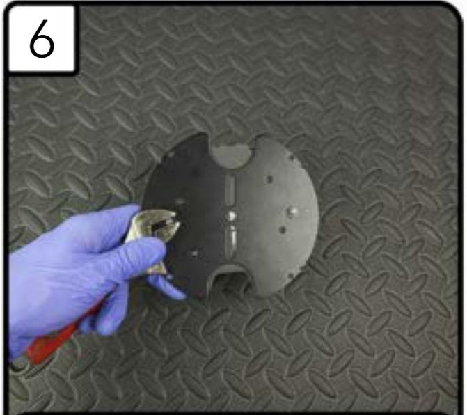
Install camera on camera mounting plate
