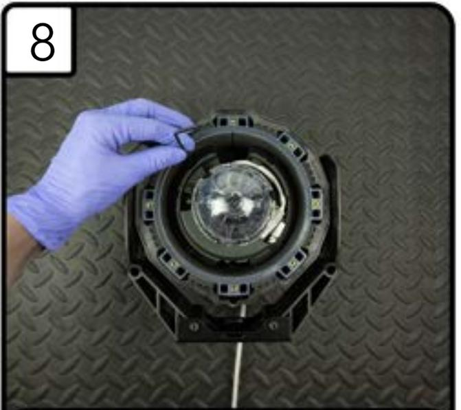
Install camera and camera mounting plate. Be sure to orient the camera mounting plate with the cutouts on the top and bottom.
