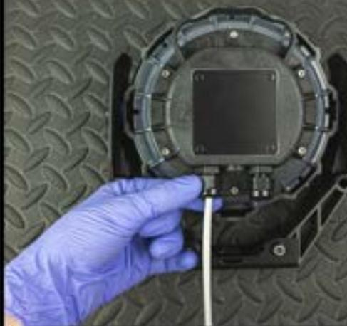
Insert power/data cables and tighten down cable gland cap
