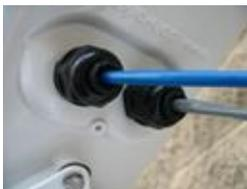
Be sure to tighten cable gland seals to assure a weather tight seal. Gently but firmly tighten four enclosure cover screws to fully seal enclosure.
