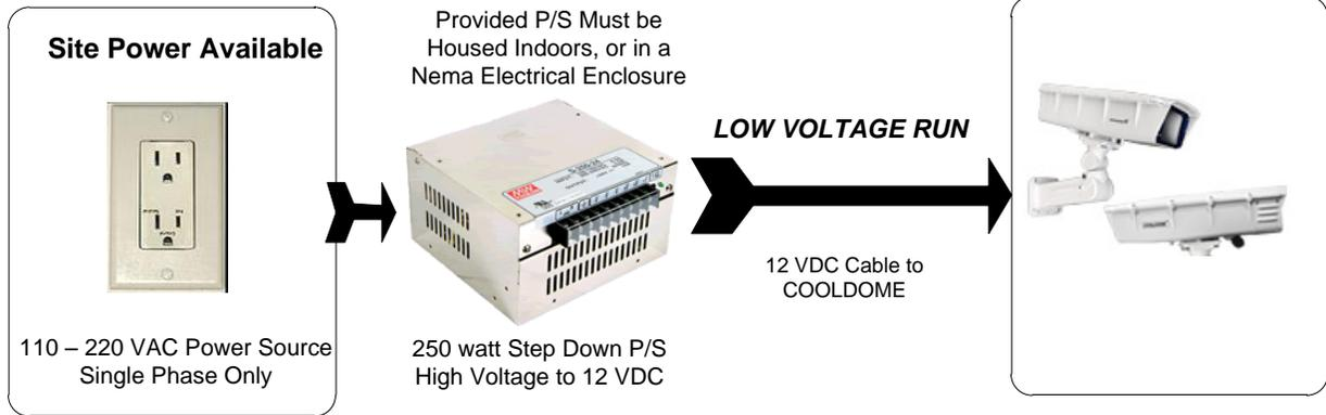
**Turn Off Power or leave power disconnected during Installation of All Wiring.
