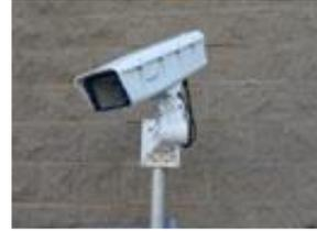
Attach housing to arm as shown, tighten screws evenly but firmly on both sides of housing. Adjust housing to desired position using both pan & tilt adjustment fasteners and tighten all bolts evenly & securely, so housing is pointing into final position.
