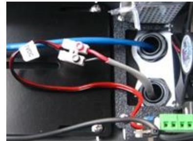
Hook up user supplied data cable to camera. Install power cable to camera. (See camera power page if your camera power cable is not compatible with the power cable shown above)
