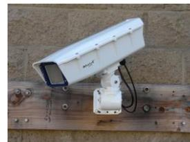
Re-assemble Housing with Pan-Tilt onto Mount Arm by securing two side screws for pan adjustment. Secure & tighten both screws evenly, also adjust & tighten tilt screws into desired final position. Be sure all fasteners are evenly and securely tightened. After completing wiring, close access door to wire feed on mount, complete internal wire & cable installation, and close and seal housing top & wire feed seals.
