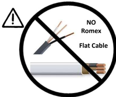
Use Round Cable Only with provide Cable Gland Port Seal
