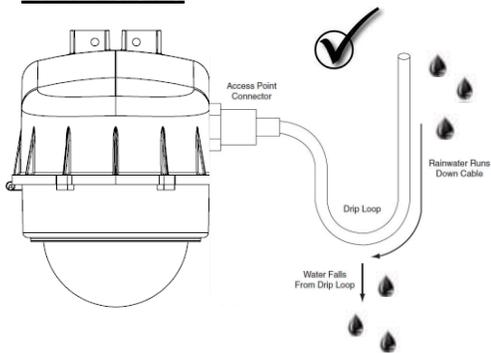
**Always Create a Drip Loop** for all Cables or Conduit Entering Dotworkz D2 Housing from level or Above D2 Conduit, Power, Data, & Antennae
