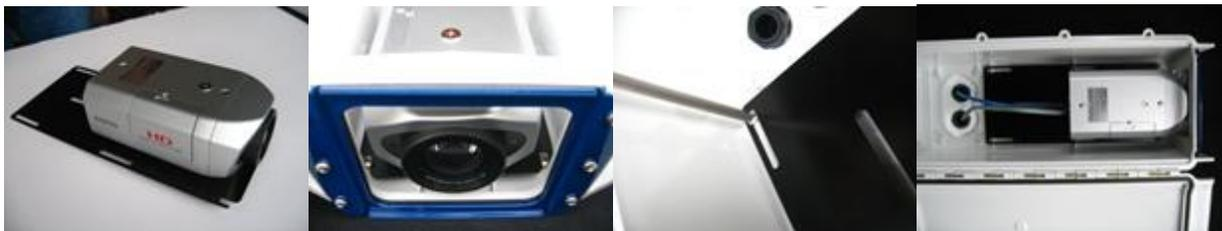
Re-install camera plate into S-Type, placing camera lens close to enclosure lens. For cameras that have adjustable focal lens', allow enough room for lens clearance. Re-install & Tighten all mounting plate screws.
