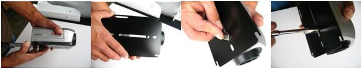
Using 1/4" bolt provided, mating camera to mount bracket. Adjust camera to sit strait and slightly overhang front of mounting bracket. Gently but securely tighten bolt with camera pointing strait on mount plate.
